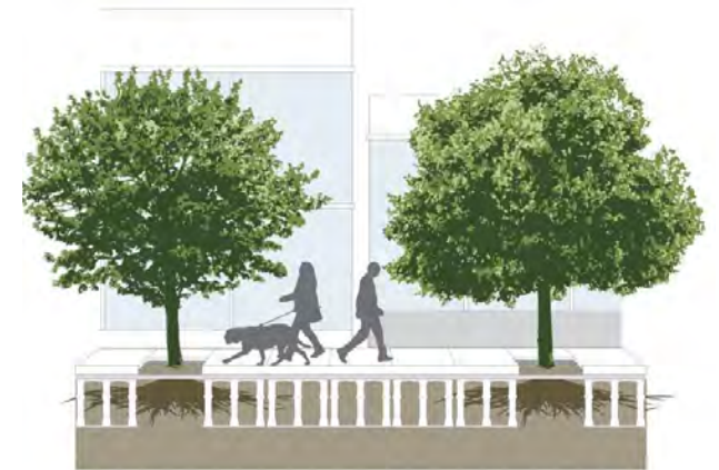
Suspended pavement systems allow for expanded soil volumes for tree roots
